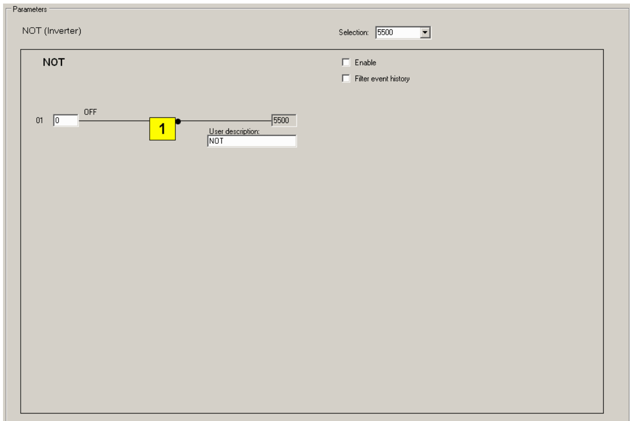
Figure 3-153 “PLC” – Logic element „NOT(Inverter)”
